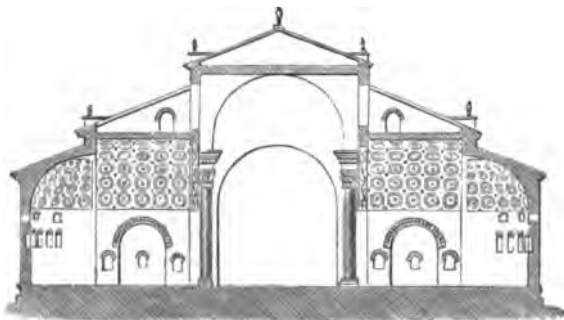
Fig. 3.—Transverse Section of Basilica of Maxentius.
